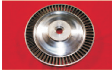
High temperature nickel based alloy turbine Ra \leq 0.2 \mu m
