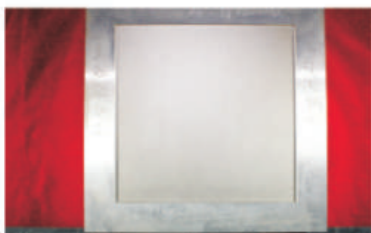
Large area machining Ra \leq 0.4 \mu m
