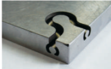
Simultaneous 4-axis machining job
