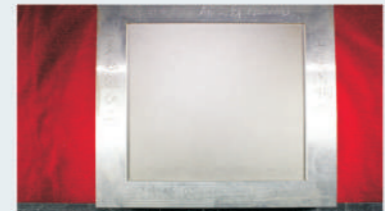
Big area machining Ra \leq 0.4 \mu m
