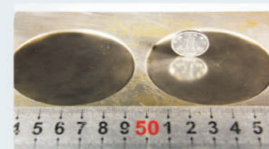
\Phi 60mm mirror finish Ra \leq 0.18 \mu m
