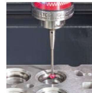
Analogue contour scan of the sealing chamfer on a valve seat
