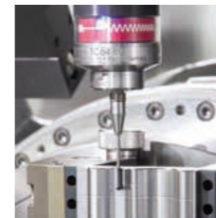
TC64-RG – Roughness measurement in the machining centre
