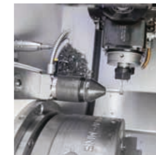
Tool measurement – TC76 with protective sleeve
