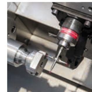
Workpiece measurement in the turning machine
