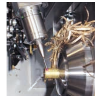
Workpiece measurement in the turning machine
