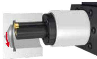
3 Cutter lifts from workpiece
