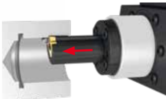
2 Cutter drives into workpiece
