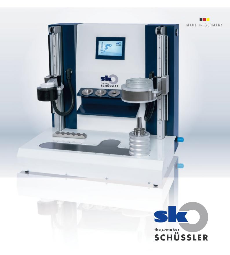
Induction coil for quick shrinking
