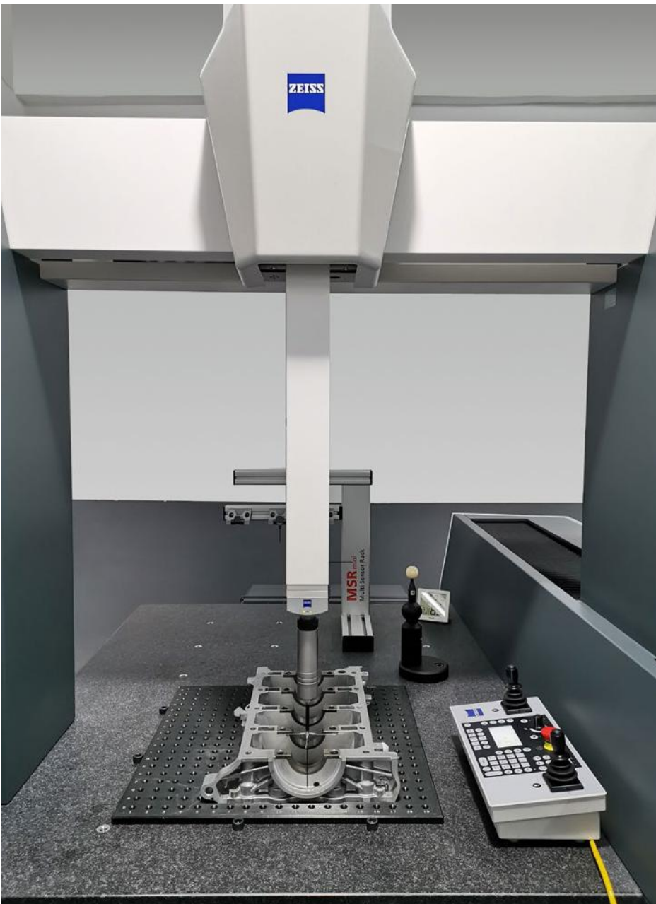
Workpiece measuring by CMM
