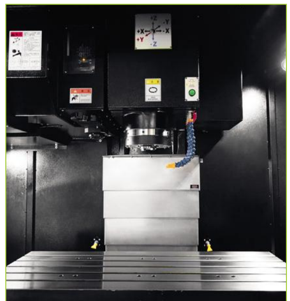
Keyarrow telescopic covers in all axes
