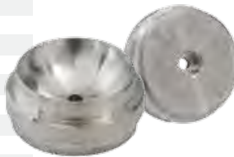
ALUMINUM - 7075-T6 - BAR STOCK CYCLE TIME: 5.40 SEC
