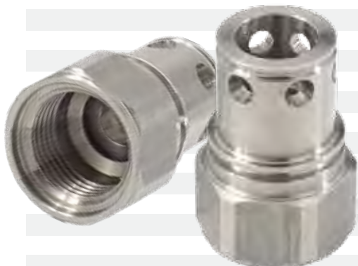
STAINLESS STEEL - 316 - BAR STOCK CYCLE TIME: 20.0 SEC
