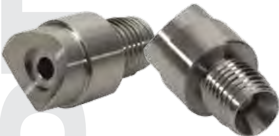
STAINLESS STEEL - 2205 - BAR STOCK CYCLE TIME: 11.9 SEC
