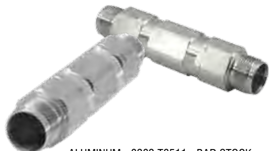
ALUMINUM - 6262-T6511 - BAR STOCK CYCLE TIME: 12.6 SEC
