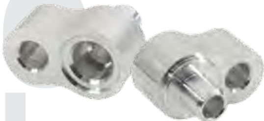
ALUMINUM - 6061-T6 - BAR STOCK CYCLE TIME: 3.5 SEC
