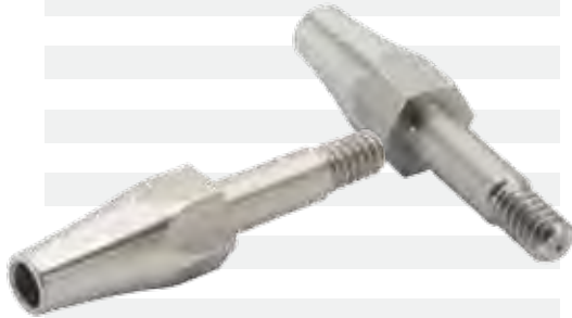
STAINLESS STEEL - 303 - BAR STOCK CYCLE TIME: 8.0 SEC
