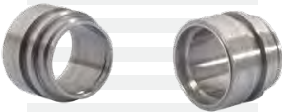
STAINLESS STEEL - 430FR - BAR STOCK CYCLE TIME: 4.2 SEC
