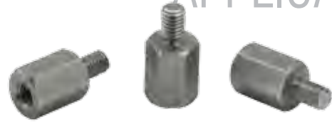
STAINLESS STEEL - 303 - BAR STOCK CYCLE TIME: 2.8 SEC
