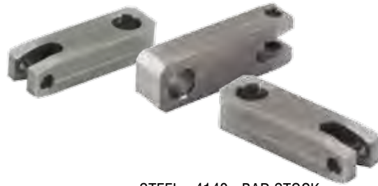
STEEL - 4140 - BAR STOCK CYCLE TIME: 10.0 SEC
