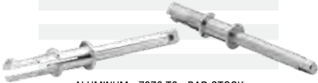
ALUMINUM - 7076 T6 - BAR STOCK CYCLE TIME: 5.8 SEC
