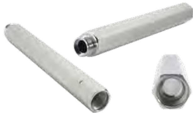
ALUMINUM - 6062 - BAR STOCK CYCLE TIME: 5.7 SEC
