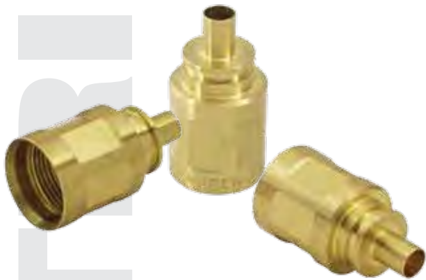
BRASS - 360 - BAR STOCK CYCLE TIME: 7.4 SEC
