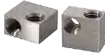
STAINLESS STEEL - 303 - BAR STOCK CYCLE TIME: 11.0 SEC
