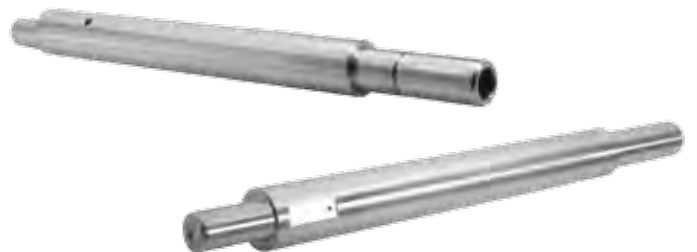
STEEL - 1117 - BLANK CYCLE TIME: 9.0 SEC
