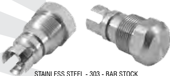
STAINLESS STEEL - 303 - BAR STOCK CYCLE TIME: 13.6 SEC
