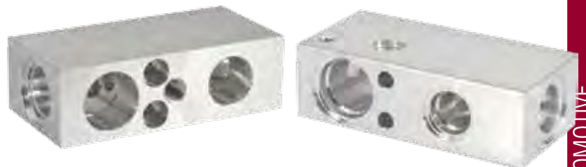
ALUMINUM - 6061-T6 - BAR STOCK CYCLE TIME: 8.0 SEC
