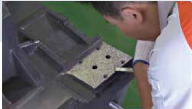
100% Hand-Scraping for Geometry Accuracy and Rigidity
